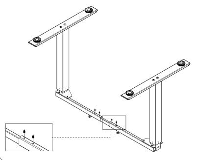
STEP 3:Insert the center rail into the frame, adjust the width and then install the frame to the center rail using four M6\*10 machine screws.
