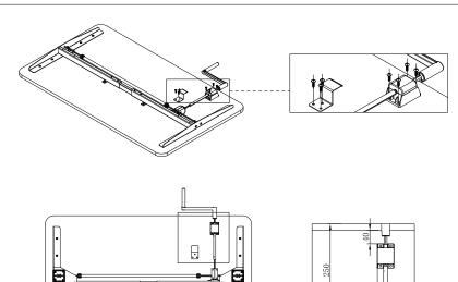
STEP 9:Install the hand crank and hand crank bracket to the table top panel using 7 ST5\*20 wood screws. (Positioning dimensions are detailed in the attached drawings)
