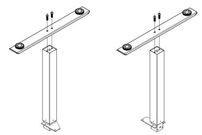
STEP 1: Install the foot to the column using four M10\*35 machine screws.
