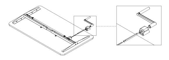
STEP 8: Insert the short drive rod into the gearbox assembly and the hand crank into the short drive rod.
