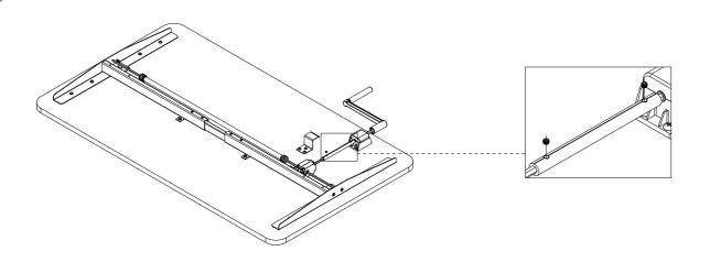
STEP 10: Lock the two M5\*4 machine screws on the short drive rod.
