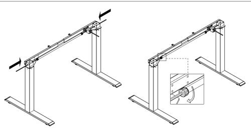
STEP 5: Tighten the knob on the long drive lever by inserting the hexagonal rod into the long drive lever from both sides.
