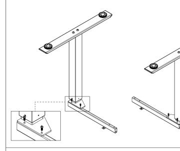
STEP 2: Intsall the column to the frame with four M6\*14 machine screws.
