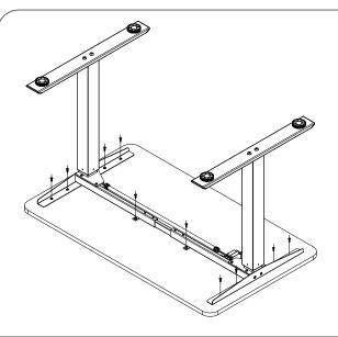
STEP 7: Install the tabletop panel to the table frame using 10 ST5\*20 wood screws.
